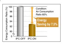
ue to estimation control, use point pressure varies in accordance with use conditions \*IPC control range of the constant speed unit is air consumption ratio of 50% or more
